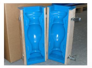
When producing a balustrade mould then make sure that the mix is as flowable as possible, this is so that the air leaves the mould as quickly and easily as possible and that the mix is compact meaning a beautiful smooth texture remains.
