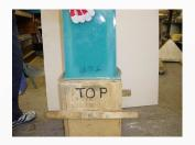
5. With carrier in upright position, place mould and concrete upside down on carrier.
