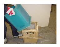
7. Concrete drops loose into carrier & mould can be removed.
