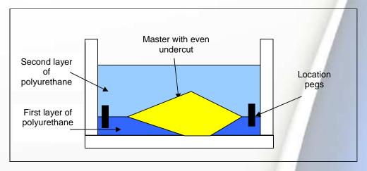
ARMCON CERTAINTY: IN CONCRETE After mould and master preparation, pour first layer of polyurethane to level of undercut on master.
