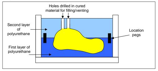
Prior to pouring the first layer of polyurethane, the released master can be suspended in the mould box or rested on spacers made from the same polyurethane as the mould making materials (spacers should be totally free of release agent otherwise they will not bond to the poured on polyurethane).
