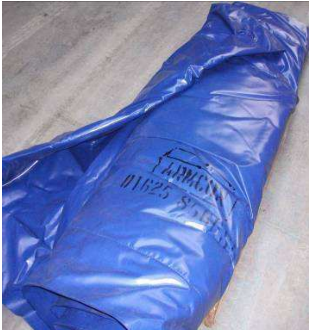
Example of a Curing blanket
